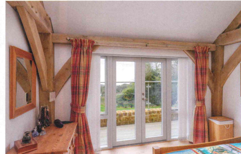
Above & left: Supplied by Rational, the frames of the triple glazed windows are aluminium on the outside and timber on the inside
