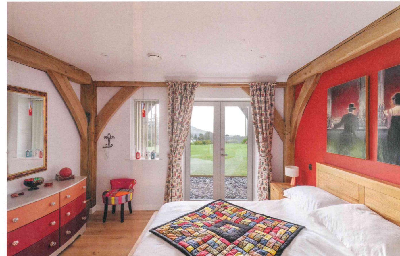
Above & left: Supplied by Rational, the frames of the triple glazed windows are aluminium on the outside and timber on the inside
